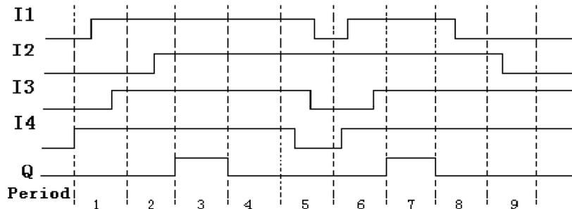
During the third period, all the statuses of the inputs are 1 and during the second period, the status of I2 is 0, so the status of the output is 1.
