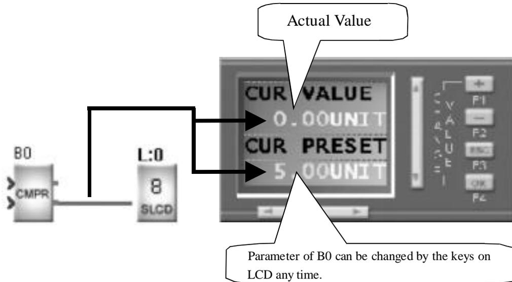
Fig. 4.4 Actual Value & Parameter of the Running
