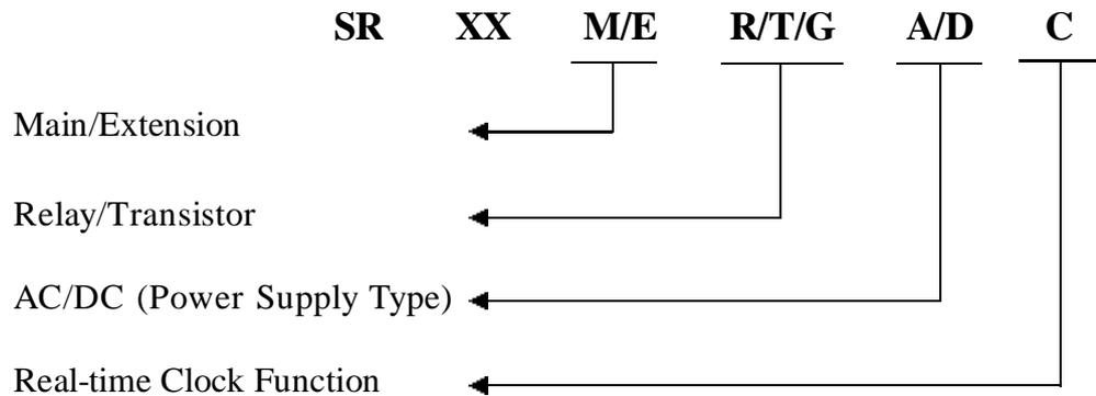
**Note:** M means main machine, E means extension module
