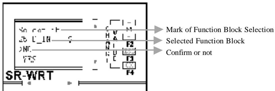
Fig. 10.8 Function Block Selection Confirmation Interface
