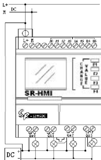
Fig. 2.12-2 The PNP Transistor Output
