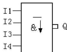
Only when the status of at least one of the input is 0 and statuses of all the inputs in the last period are 1, the output status of this NAND with RLO borderline test is 1.
