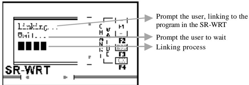
Fig. 10.18 Process Interface of Linking to SR-WRT
