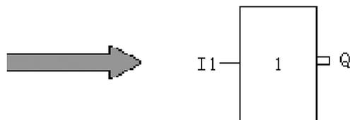
This function block is called NOT, because if the input status is 0, then output Q is 1, and vice versa. In other words, NOT is the phase inverter for the input point.
