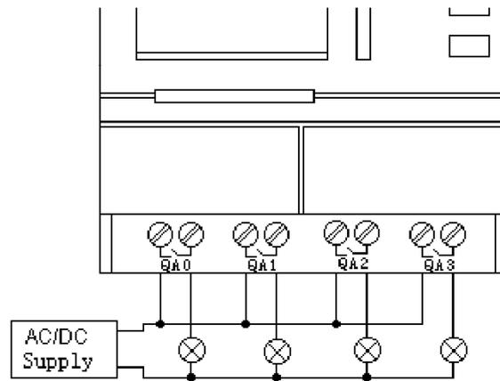
Fig. 2.11 Relay Output
