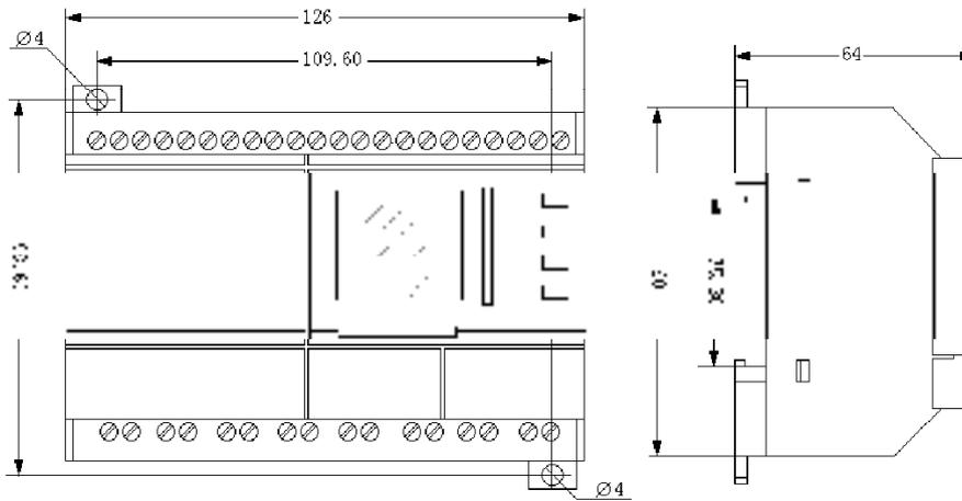
Fig. 2.3 Installation Dimension of SR-22 Series (mm)
