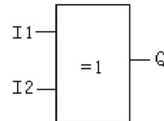
When the statuses of all the inputs are not the same, the output status of XOR is 1.
