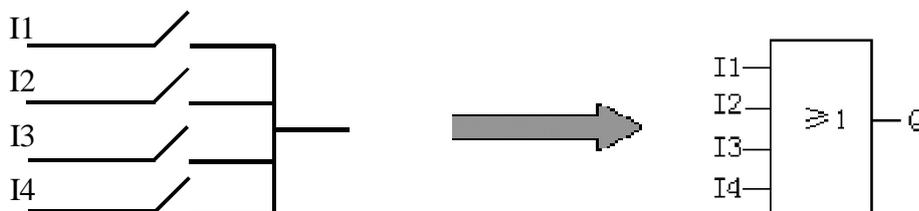
This function block is called as OR, because the status for at least one of the inputs I1, I2, I3 or I4 is 1 (i.e. closed), then output Q is 1.
