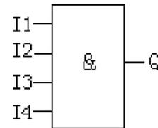
This function block is called AND, because only when all of I1, I2, I3 and I4 are all in status 1, the status of Output Q will be 1 (i.e. the output is closed).
