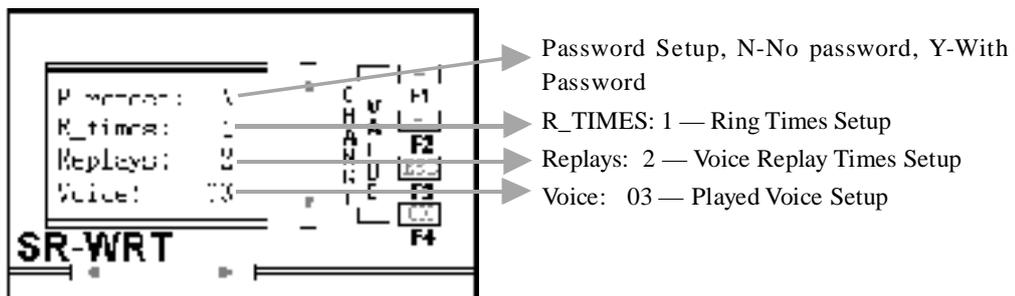
Fig. 10.36 Voice and Relative Parameter Setup Interface
