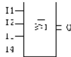
In NOR function block, when the statuses of all the inputs are low potential (status 0), then the output is connected (status 1). If the status of any input is high potential (status 1), then the output is opened (status 0).
