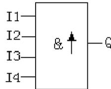
Only when all the statuses of the inputs are 1 and at least the status of one input is 0 in the last period, the output status of AND with RLO borderline test is 1.
