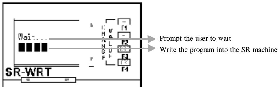
Fig. 10.19 Process Interface of Writing Program into SR
