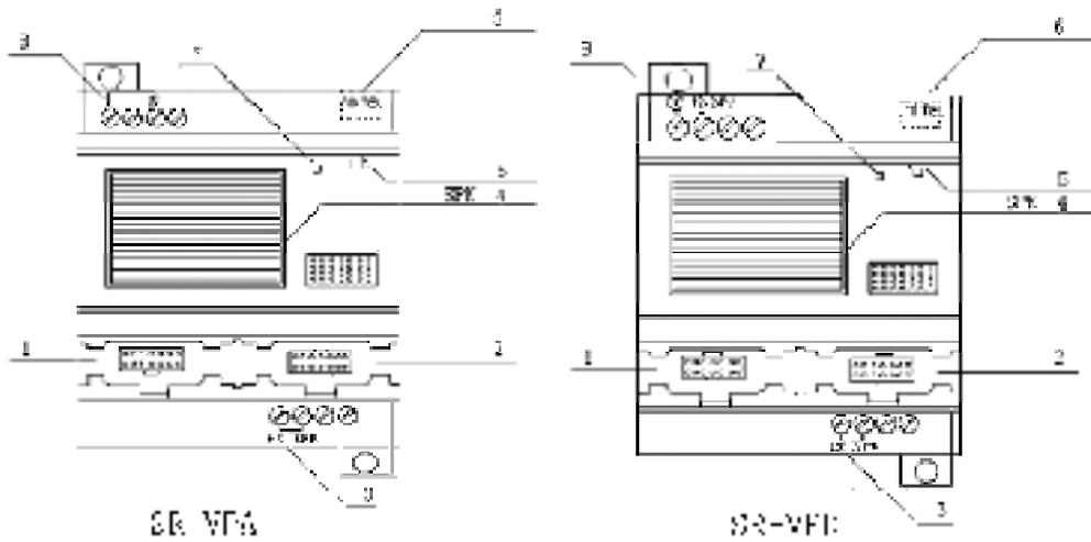
Fig. 5.1 Structure of SR-VP Series Voice Module
